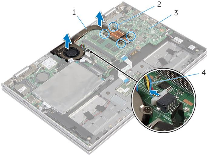
1 processor fan and heat-sink assembly
