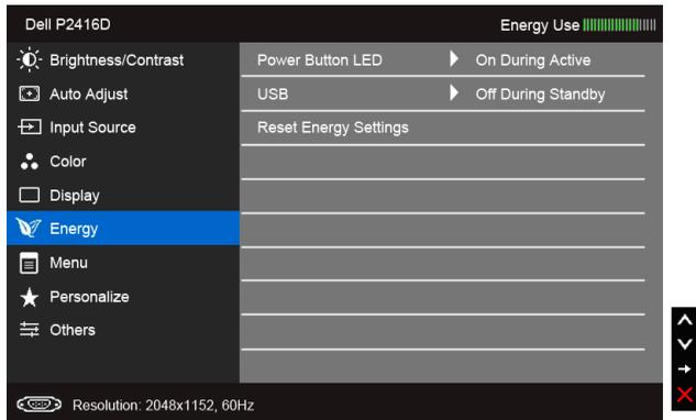
**Power Button LED** Allows you to set the power LED indicator On or Off to save energy.
