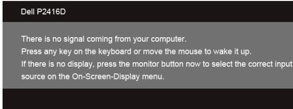
If either VGA, HDMI, or DP input is selected and the corresponding cable is not connected, a floating dialog box as shown below appears.
