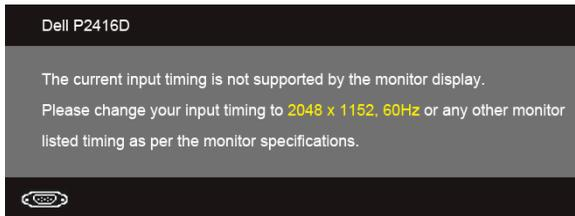
This means that the monitor cannot synchronize with the signal that it is receiving from the computer. See [Monitor Specifications](#) for the Horizontal and Vertical frequency ranges addressable by this monitor. Recommended mode is 2560 x 1440 (for HDMI/DisplayPort) or 2048 x 1152 (for VGA).
