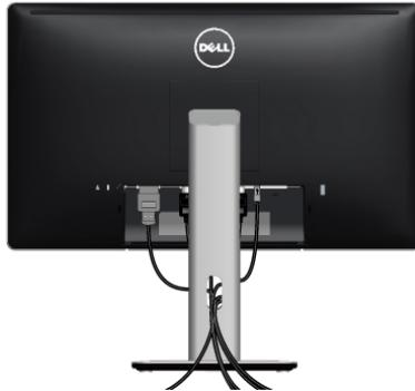
After attaching all necessary cables to your monitor and computer, (See [Connecting Your Monitor](#) for cable attachment,) organize all cables as shown above.
