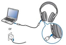
The Charge/NC indicator blinks during charging. It takes approximately 3 hours to charge the headphones. (The duration time differs depending on the charging output.)
