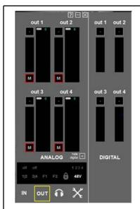
Click on the icon on the bottom right of the "ANALOG" window, to view the digital level on the outputs signals. A vumeter is displayed for each input channel, which gives the digital level of the signal on the digital output, expressed in dBfs (0dBfs is the maximum value of a digital sample).
