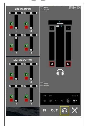
Click on the icon on the bottom left of the central headphones window to access the DIGITAL OUTPUT section, for adjusting the levels of the signals played on the AES/EBU outputs from a software application.
