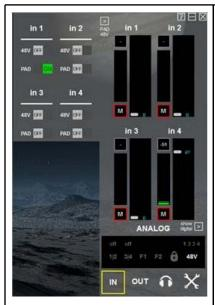
Click on the icon on the top left of the ANALOG panel to display the panel allowing to set Pad and 48V on the inputs.
