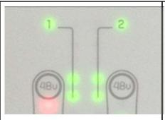
In case you are using a static microphone on an analog input, it is necessary to activate the 48V phantom power on this input.
