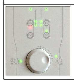
Pressing the button several times allows selecting analog output 1, analog output 2, both outputs, or no output (LED turned off).
