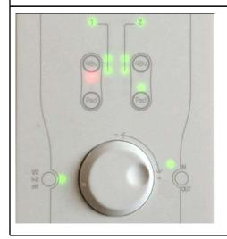
Pressing the button several times allows selecting analog input 1, analog input 2, both inputs, or no input (LED turned off). The analog gain adjustment is then applied to
