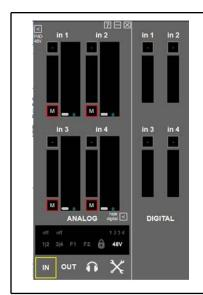
Click on the icon show on the bottom right of the "ANALOG" window, to view the digital level on the inputs signals. A vumeter is displayed for each input channel, which gives the digital level of the signal on the digital input, expressed in dBfs (0dBfs is the maximum value of a digital sample).
