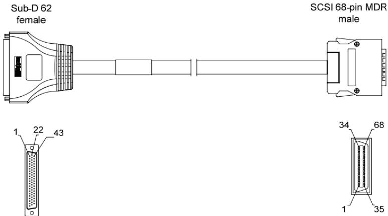
If you dispose of a VX1221<sub>HR</sub> or VX1222<sub>HR</sub> cable, this adapter allows its use with the VX PCI EXPRESS™ multichannel boards.
