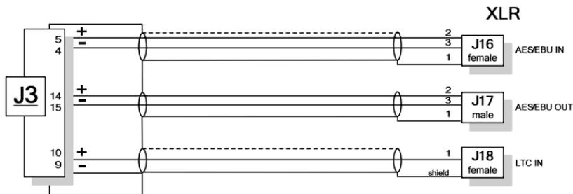
**Note:** digital cable for VX222HR with additional AES/EBU Sync input on special request.
