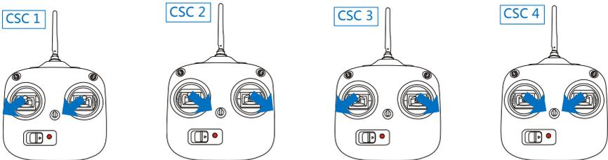
Under the conditions stated below, the motors will stop in ATTI. Mode/GPS ATTI. Mode:
