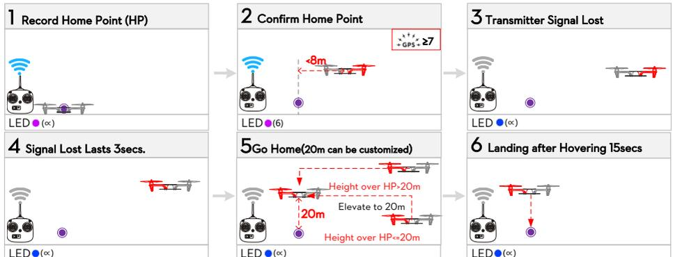
(1) The aircraft will not go home (only attitude stabilizing) in the condition that  $\text{GPS} < 6$  or GPS is not working, even if Transmitter signal is lost or Go Home switch is triggered.
