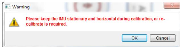
Place the IMU on a stationary and horizontal surface and ensure A2 logo faces upward.
