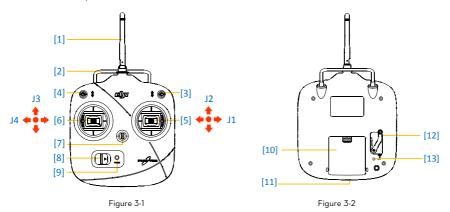
[1]Antenna [2]Carrying Handle [3]3-Position Switch S1 [4]3-Position Switch S2 [5]Joystick1(J1;J2) [6]Joystick2(J3;J4) [7]Neck Strap Attachment [8]Power Switch [9]Power Indicator [10]Battery Compartment [11]Micro-USB Port [12]Slide Lever [13]Potentiometer
