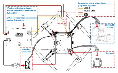
The diagram below illustrates the conneciton between the iOSD Mark II and the wireless video transmission module.
