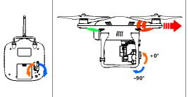
Slide Lever controls the pitch of the H3-2D and H3-3D gimbal. The position of slide lever determines the pitch angle relative to the horizontal level.
