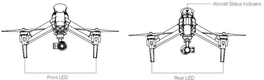
The Front and Rear LED show the orientation of the aircraft. The Front LED displays solid red and the Rear LED displays solid green.
