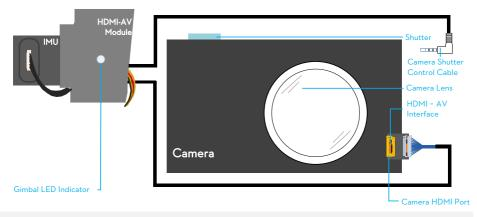
stepl: Connect the gimbal HDMI-AV module to camera HDMI port with a HDMI-AV connection cable.
