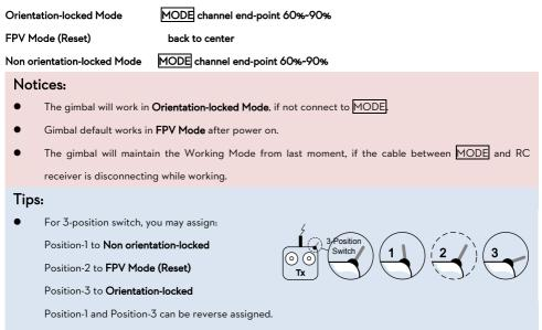
• One 2-position switch can be assigned for any two of the working modes as you like.
