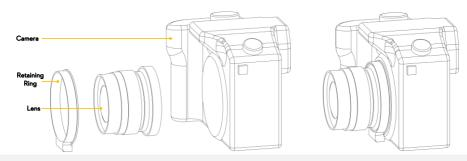
stepl: Mount the lens onto the camera first, and then put the retaining ring through lens until it is fixed.
