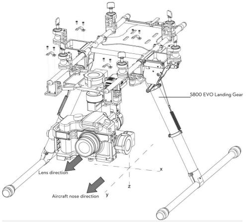
step4: Install the gimbal to a landing gear with mounting bracket; tighten up the screws (2.5\*8 Head-cup screw×8) with appropriate screw glue.
