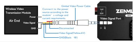
**stepl:** Carefully solder the corresponding Video Signal/GND cables to a wireless video transmission module (Air End).
