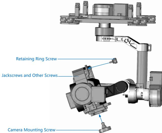
**Step4:** Mount the camera into the gimbal and tighten the camera mounting screw.
