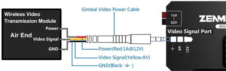
**Step1:** Respectively solder the Power/Video Signal/GND cables to wireless video transmission module (Air End).
