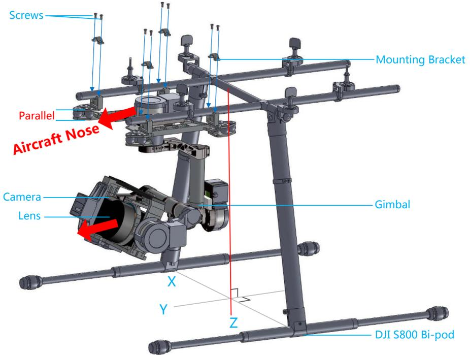
**Step7:** Install gimbal to a bi-pod with mounting bracket; tighten up screws (2.5\*8 Head-cup screwx8) with appropriate screw glue.
