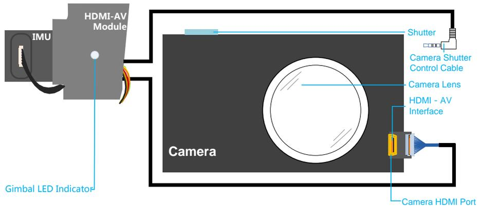
**Step1:** Connect the gimbal HDMI-AV module to camera HDMI port with a HDMI-AV connection cable.
