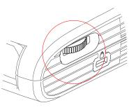
■ The focus adjustment can be performed when the throw distance is between 48cm and 133cm.
