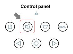
Press the " < >" buttons on the control panel to controlling the volume.
