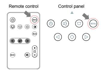
The menu will be closed if the MENU button is pressed again. The menu will also be closed automatically after 30 seconds of no operation.
