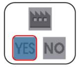
Press the  $\checkmark$  button to execute the selection. Select "YES" to return to factory default settings. When configuration is completed, the screen returns to start menu.
