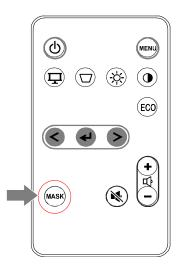
Press the MASK button again to return to the input signal screen.
