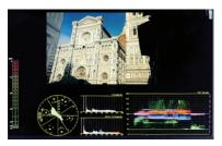
All Scopes: Display all the scopes in the Scopes menu (Histogram, Audio Column, Vector, RGB Histogram, and YUV Waveform) on the sides of the frame with an uninterrupted view of your incoming video image. The default setting is Off. You can also add the scopes individually to display them over your image.
