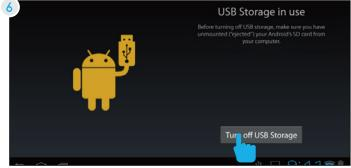
Before turning off USB storage, make sure you have unmounted ("ejected") the FunTab pro and SD card from your computer. Tap Turn of USB Storage.
