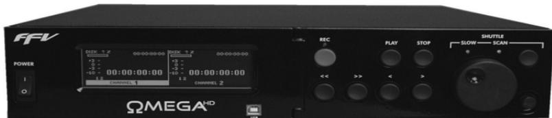
**POWER:** Switch that turns the unit on / off. Please allow at least 30 seconds after turning the unit on for it to boot-up and recognize the disk.
