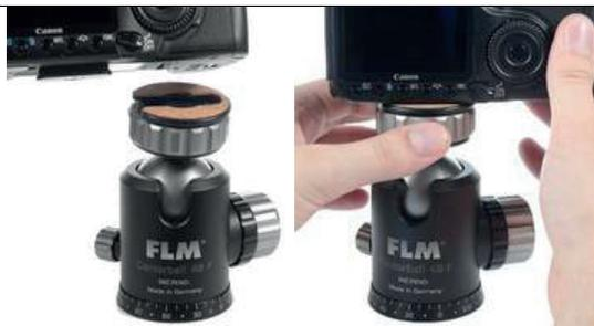
The plate, which is screwed on, is shoved laterally into the Power-Release Basis. The basis is offered with a diameter of 45 mm and 55 mm. For the larger version, a camera plate with pin is available and this prevents the twisting of the plate.
