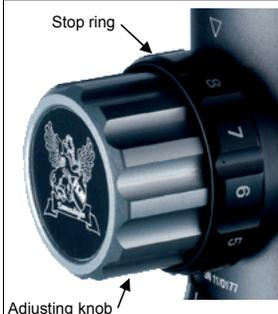
First rotate the stop ring counterclockwise and then the adjusting knob counterclockwise to the outmost stop. Now, you can easily move the ball with your hand.
