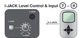
This stereo mini jack input (8) is designed for connecting portable music players. This is a stereo unbalanced input with approximately 10k Ohms input impedance.
