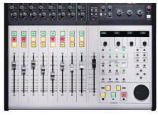
The 8 Fader Strips (faders, **SEL**, **CUT** & **SOLO**) flip between controlling analogue channel levels and track faders within the DAW. This dual-layer technology makes it easy to switch from analogue to DAW control in an instant.
