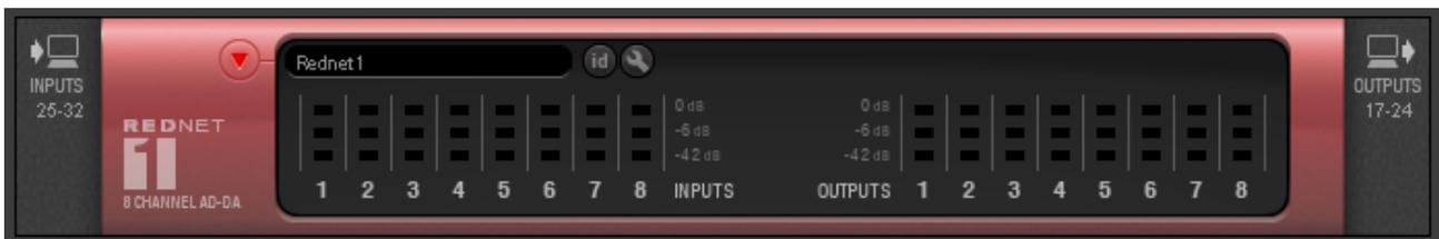
**Metering:** Each input and output has 3 virtual LEDs corresponding to the levels indicated by the tricolour LEDs on the physical front panel. These illuminate at -42 dBFS, -6 dBFS and 0 dBFS respectively.
