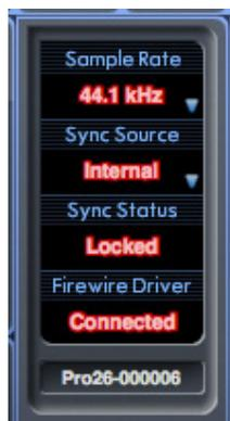
The Device Status section displays the current sample rate, synchronisation source and sync and driver statuses of the Saffire PRO 26. Sample rate and external synchronisation source can also be set, permitting the Saffire PRO 26 to be used with other digital devices.
