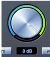
Set the level of all assigned outputs (see 'Blue' on page 26) with this rotary control. Note that the physical **MONITOR** control on the Saffire PRO 26's front panel must also be "turned up" for audio to be heard from Line Outputs 1 & 2; the hardware and software monitor volume controls are effectively "in series" for these outputs. The dB display below shows the current level to which the monitor knob is set.
