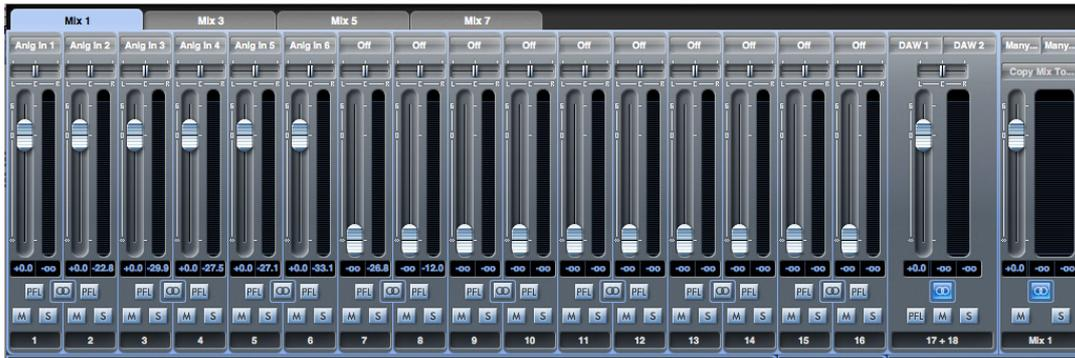
Saffire MixControl includes a total of 8 mixes, each with a maximum of 18 channels in the mix. Up to 8 mono mixes or 4 stereo mixes, (or any combination of mono and stereo mixes) are available, making up a total of 8 mix channels.
