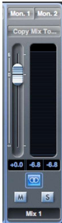
The signals in the mixer's input channels are summed (mixed together) and routed to the mix's output channel. The output channel lets you control the overall level of the entire mix.
