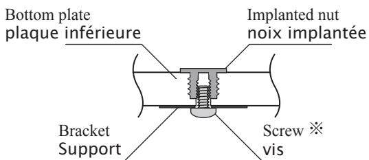
※ Recommended screw length (thickness of bracket: 1mm)
