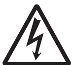
The lightning flash with arrowhead symbol, within an equilateral triangle, is intended to alert the user to the presence of non-insulated "dangerous voltage" within the product's enclosure that may be of sufficient magnitude to constitute a risk of electric shock to persons.
