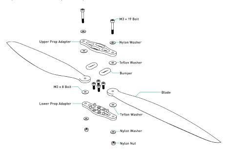
To reassemble, follow the part layout in the figure above. Note that there are two different types of washers, one made of nylon and the other made of PTFE. The nylon washer is smaller in width and thicker and is installed between the nut or bolt head and the two prop adapters. The PTFE washer is wider and thinner and is installed between the prop blades and prop adapters.
