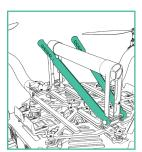
**4.** Place battery pack(s) on battery tray below handle
