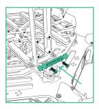
2. Adjust battery stops to fit battery pack(s)
