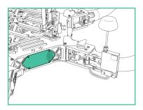
7. Zip tie the FPV transmitter lead to the boom cable bundle for strain relief.
