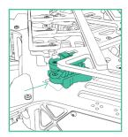
To install, place the cartridges between the top chassis plate and the battery plate. Ensure they are engaged in the track features and are parallel with the chassis and battery plate. Push inwards fully until they click, indicating the cartridges are locked in place. Pull outwards on the cartridge to ensure it is locked in place.
