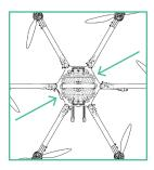
2. Remove side closeout panel with radio wires using a 1.5mm hex driver
