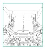
**5.** Tension and secure battery retention straps
