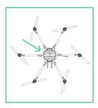
2. Remove the side closeout panel with the jumper using a 1.5mm hex driver
