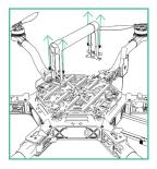
**4.** Attach the supplied Toad to the top plate using the four M3×8 bolts provided
