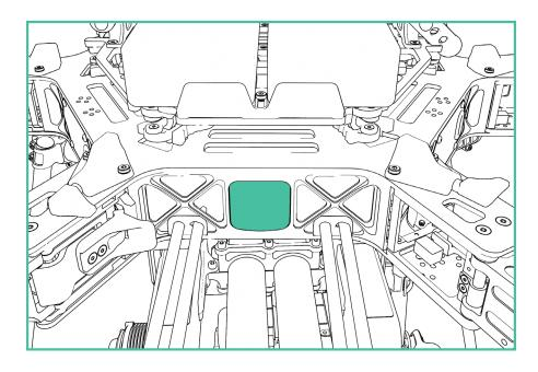
The rear-facing Status Light shows the status of ALTA as it boots, arms and flies. The following table shows the different meanings of the light in the various flight phases.
