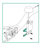
2. Attach Accessory Mount to boom 5 with M3×8 flathead bolts.
