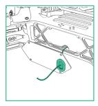
**4.** Connect the white connector to the external voltage sense port on the Futaba receiver.
