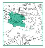
To remove, pinch the cartridge latch to unlock it from the battery and chassis plate. Simultaneously pull the battery and chassis plate apart while pulling the cartridge outward.
