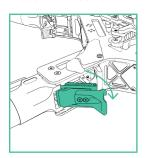
**4.** Fold up all six boom retention clips to secure booms
