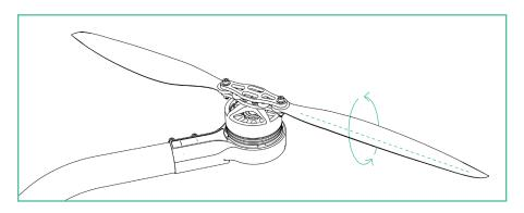
Over time, the bolts that hold the propeller blades to the prop hub can loosen due to vibration. To check prop bolt tightness, twist the prop about its length. If there is free play, the prop bolt is too loose. Use the provided 2.5mm hex driver and wrench to tighten the bolt and nut that secure the prop blade just enough to remove the play.
