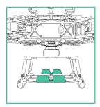
**2.** Attach the single-hole end of the battery retention strap to a stud on the landing gear
