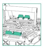
3. Attach the single-hole end of the battery retention straps to the studs
