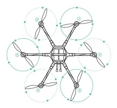
Propeller blades should be removed when making a change to the configuration of the ALTA to prevent propeller strikes in the event of unintentional motor starts and should be replaced on an as needed basis if they become damaged. Generally, a nick on the leading edge that is large enough to catch a fingernail indicates that the prop should be replaced. If the blade composite structure becomes delaminated, the propeller blade should be replaced.
