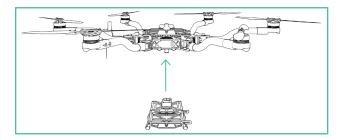
3. Remove the four flat-head M3×6 bolts that secure the top handle
