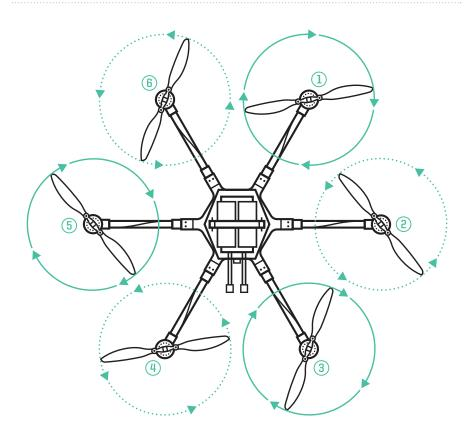
The folding propellers include two carbon fiber propeller blades attached to prop hubs, which are themselves secured to the motors. The propellers installed on booms 1, 3 and 5 spin clockwise when viewed from above ALTA, and the propellers installed on booms 2, 4 and 6 spin counterclockwise when viewed from above.
