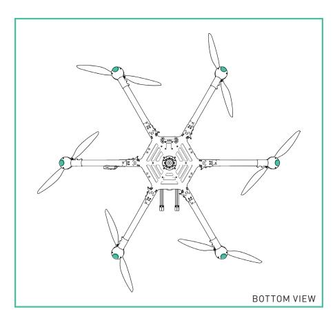
The boom-end mounted Orientation Lights indicate both the orientation of ALTA in flight and the status of the individual motor Electronic Speed Controllers (ESCs) during other flight phases. The following table shows the different meanings of the light colors in the various flight phases.
