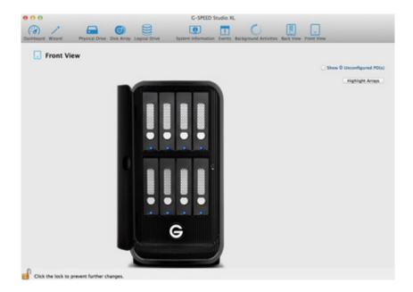
Click on the drive modules to view the status and identify the assigned disk array.
