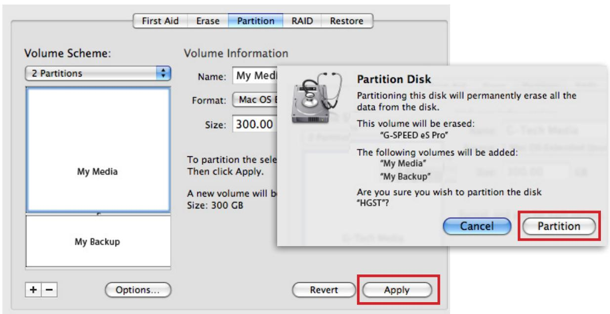
8. Click on the Partition button to continue. A Progress bar in the lower right corner of the window will show you the Progress of the disk's reformatting.
