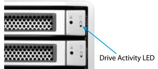
**NOTE:** It is possible the failed drive will be completely offline. In this case, the drive's Activity LED will be completely turned off, indicating the failed drive.
