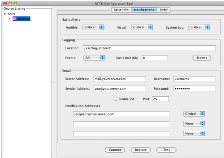
The ConfigTool has four types of Alerts: Audible Alert, Visual Alert, System Log and By Email. You can set the Event threshold for each Alert type and for different email addresses. To enable email notification, enter your server information and up to three recipient addresses.
