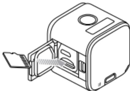
**NOTICE:** Use care when handling memory cards. Avoid liquids, dust, and debris. As a precaution, power off the camera before inserting or removing the card. Check manufacturer guidelines regarding use in acceptable temperature ranges.
