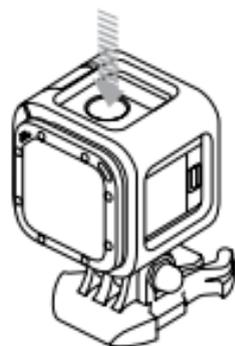
**PRO TIP:** When carrying your camera in a bag or pocket, place the camera upside down in a frame (with the **Shutter/Select** button [
