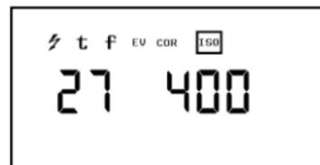
Once the film speed has been set, it is transferred to the memory of the SIXTOMAT F2 and maintained when the meter is set to any operation function. It remains visible on the top right-hand side in the digital display.
