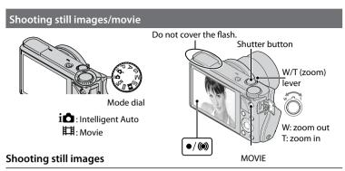
**1** Press the shutter button halfway down to focus. When the image is in focus, a beep sounds and the ● or (●) indicator lights.
