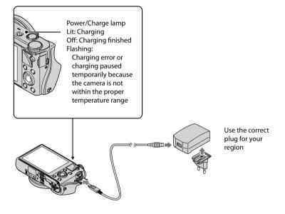
**1** Connect the camera to the AC Adaptor (supplied), using the micro USB cable (supplied).
