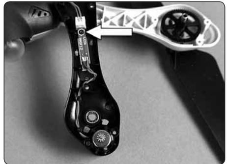
1. Remove the landing gear below the arm with the defective motor.
