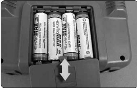
1. Install 4 AA batteries in the transmitter by removing the battery cover from the back of the transmitter. Double-check the polarity of each battery before replacing the battery cover.
