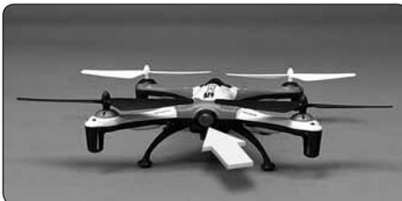
1. Turn on the TX465 transmitter and lay it down near the quadcopter on a level surface. When the display shows 000, connect the battery but do not move the quadcopter. When the Status LED is steady, the 230Si can be picked up.
