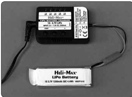
1. Plug the wall power supply into any 110V standard outlet. Plug the 4mm plug into the side of the charger box. The center front panel LED will light letting you know the charger has power. Connect the battery to the charger and it will beep twice, letting you know the battery is connected.
