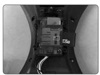
To minimize any chance of data being lost on the microSD card, do not insert or remove the card from the camera until the battery has been unplugged from the quadcopter. Remove the microSD card from the protective case. Flip the 230Si over and push the card into the slot on the side of the camera module. When the card is correctly installed, it will click. To remove the card, simply press
