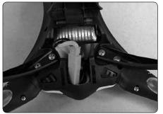
2. Slide the battery into the battery compartment, tuck the wires into the opening, and close the battery cover. When you are ready to take off, place the quadcopter on a level surface and the LED to be steady "ON". This allows the TAGS-FX control board to calibrate.
