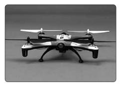
Remove the screw holding the rotor blade to the motor shaft and pull the blade up to remove it. There are arrows on the rotor blade and arm indicating which direction the rotor blade will rotate. When installing the rotor blades on the 230Si, please select a blade the same color and with an arrow in the same direction.
