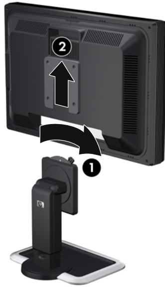
Figure 3-11 Removing the Monitor from the Pedestal Base
