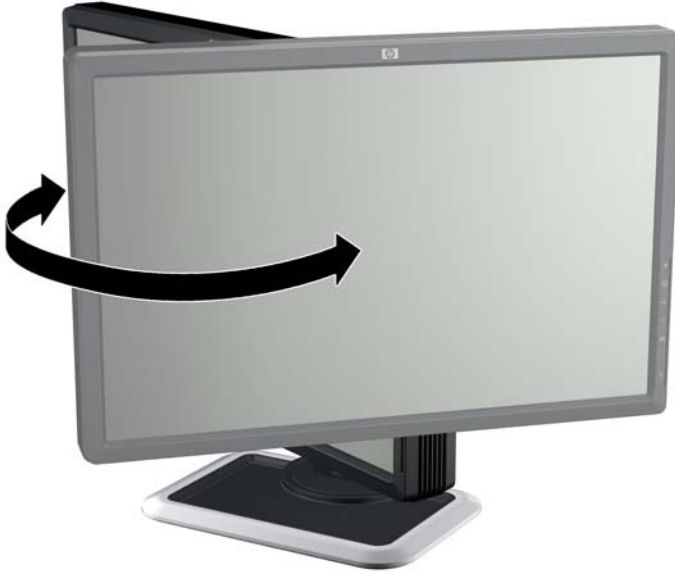
Figure 3-7 Swiveling the Monitor
