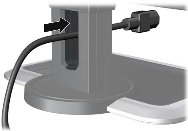
Figure 3-3 Using the Cable Management Feature
