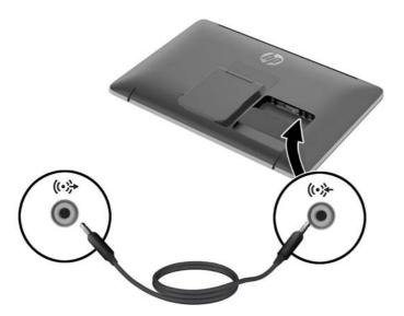
6. Plug the round end of the power supply cord into the power supply connector on the rear of the monitor (1). Plug the power cord into the power supply brick (2) and connect the other end of the power cord to an electrical outlet (3).
