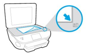
**f.** Follow the instructions on the printer display to align the cartridges. Recycle or discard the cartridge alignment sheet.
