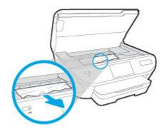
CAUTION: If the paper tears when you are removing it from the rollers, check the rollers and wheels for torn pieces of paper that might be remaining inside the printer.
