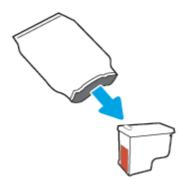
**b.** Remove plastic tape using the pull tab.
