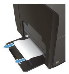
2. The jammed sheet may also be accessible by removing Tray 2 and removing the jammed sheet by pulling it to the right and then out of the product.
