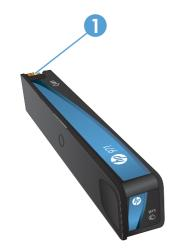
1 Metal connector and ink nozzle. Do not touch. Fingerprints may cause supply error messages. Dust may also cause supply error messages; do not leave ink cartridges outside the product for prolonged periods of time.
