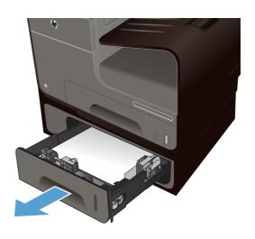
Remove the jammed sheet by pulling it to the right and then out of the product.
