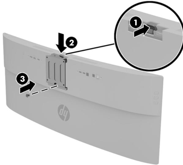
4. To attach the monitor to a swing arm or other mounting device, insert the four supplied mounting screws through the holes on the mounting device and into the screw holes on the VESA mounting bracket.
