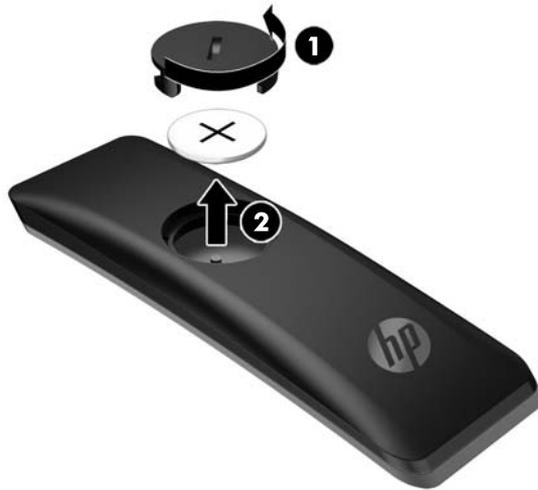
2. Install the new battery in the battery compartment with the positive side facing up (1), and then replace the battery cover (2).
