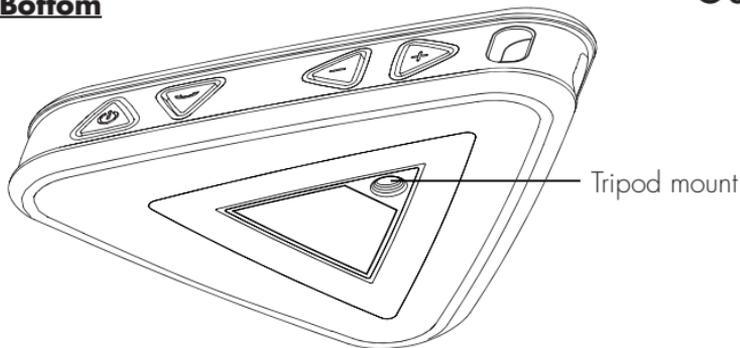
The threaded tripod mount on the bottom of the iBT3 allows you to mount the unit to a bicycle mount (not included, visit [www.ihome.com](http://www.ihome.com) to purchase) for sound on the go. To do so, screw unit clockwise onto camera/tripod mount.
