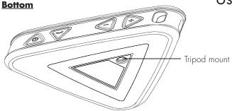
The threaded tripod mount on the bottom of the iBT3 allows you to mount the unit to a bicycle mount (not included, visit **www.ihome.com** to purchase) for sound on the go. To do so, screw unit clockwise onto camera/tripod mount.
