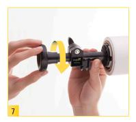
Insert the other expandable core into your paper roll and tighten its fit by rotating the control knob clockwise.
