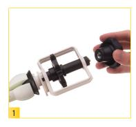
Unscrew and remove the chain drive control knob.
