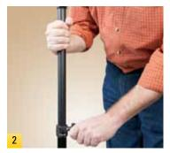
Raise the height of the stand by unlocking the sections. Start with the lowest knob, and raise each section to your desired height. Re-tighten each knob.
