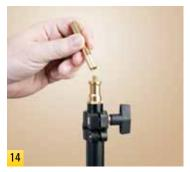
You can unscrew the 3/8" spigot tops from the support stands and use the 1/4"-20 and 5/8" studs to mount lights or other lighting equipment. Don't lose the spigot!
