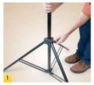
Start with one of the stands. Unlock the legs by turning the knob counter-clockwise. Spread the leg sections, but maintain a low center of gravity. Re-tighten the knob.
