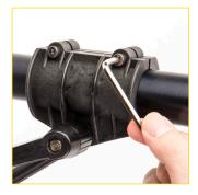
Note: If tightening the ratchet handle does not securely lock the position of the boom arm, you may use the included Allen key to tighten the two Allen screws in the base riser collar. This will lock the position securely. To change the position of the boom arm again, you will have to first loosen the Allen screws.
