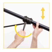
To raise or lower the boom arm, loosen the ratchet handle and push the boom arm up or down to the desired position. Lock the position by hand-tightening the ratchet handle.
