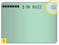
Press the Menu Dial until the screen displays only the top menu bar as shown above. Note the speaker symbol in the top right corner.
