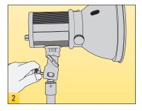
Adjust the tilt of the light by loosening the tension knob on the side and re-tighten when a suitable angle is found.
