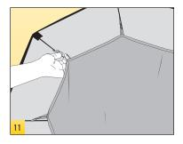
Stretch the diffuser over the edge of the OctaCool softbox. Make certain that the diffuser fits tightly on all sides.
