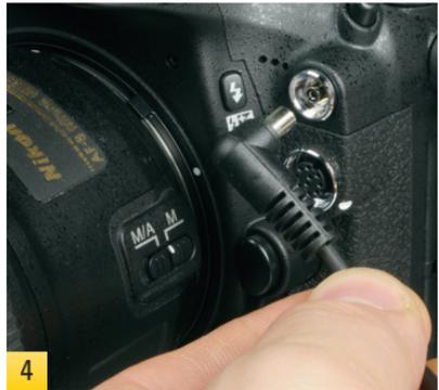
Plug the other end of the sync cord into your camera's PC terminal. Your Slave Flash will now fire immediately when you trigger your camera's shutter.
