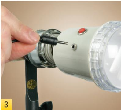
Plug the 3.5mm miniplug end of the included PC sync cord into the sync terminal on the side of the SF-AE56. The sync terminal is located on the back of the SF-AE80.
