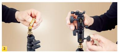
Some light stands have a threaded screw on top. If the stud is  $5/8^{\circ}$  in diameter below the threads, you may wish to mount your bracket directly to this stud. If the screw is  $3/8^{\circ}$  or 1/4," use the removable brass mounting stud adapter. Screw the brass adapter onto the threads of your light stand and mount the umbrella bracket as shown in step 2.
