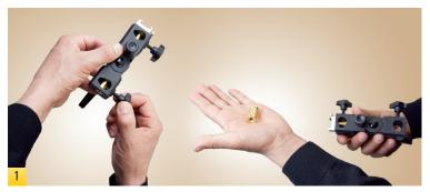
The Standard and Deluxe Umbrella-Mount brackets are very similar, but we'll show how to set up both models in this guide. Begin by loosening the locking knob. Remove the brass mounting stud adapter. Even if you don't need this stud adapter for your current setup, don't lose it. You may need it in the future.
