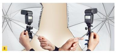
The umbrella socket slopes upwards slightly to give your flash better beam spread into your umbrella. Insert the umbrella shaft into the high end of the umbrella socket and tighten the thumbscrew. Don't over-tighten, to avoid pinching the umbrella shaft. Umbrellas larger than 45" are not recommended for use with these brackets.
