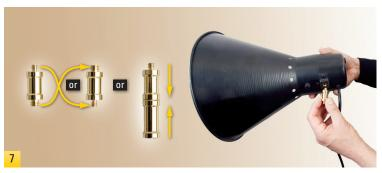
To mount a small light fixture, unscrew and remove the cold shoe. Mount the light using the exposed  $1/4^{\prime\prime}$  screw. Or turn this fitting around for the  $3/8^{\prime\prime}$  screw. If you need a  $5/8^{\prime\prime}$  stud fitting, connect the two brass fitting adapters. This gives you a standard  $5/8^{\prime\prime}$  stud fitting that most lights use.
