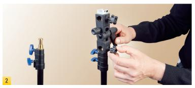
If your light stand has a standard  $5/8^{\circ}$  stud on top, mount your bracket on the stud and tighten the locking knob.
