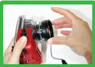
4. Position filter so that it is "square" and evenly placed on lens port ring.
