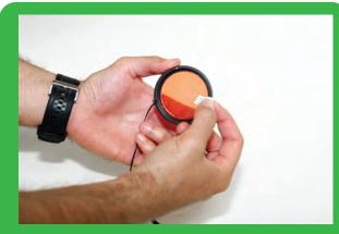
2. If installing a new filter, remove protective film from front and back of filter.
