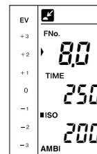
Move measuring parameter indicator to ISO position by pressing DISP button. After you input required f-number and shutter speed, ISO will be measured and displayed digitally according to input data.
