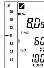
The f-number corresponding to the shutter speed set in step 4 is displayed on the digital readout as well as on the analog scale with a pointer ( — ). The proportion of flash light illuminating the composition is shown on the analyze scale.
