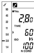
Two quadrants are lit up on the display, indicating that the proportion of flash light is approx. 50% (ambient: flash ratio = 1:1).
