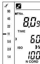
The f-number corresponding to the shutter speed set in step 3 is displayed on the digital readout as well as on the analog scale with a pointer (—).
