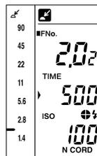
This simulation is based on controlling the ambient light by varying the shutter speed. The proportions of ambient light and flash light can also be adjusted by changing the intensity of the flash light. The intensity of flash light can be controlled either by varying the distance between the subject and the flash, or by changing the power (light output) of the flash.
