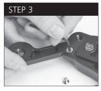
3. Attach ARM BRACKET (i) to the bottom of the BASE PLATE (c) with (2) 10 – 32 x 1/16" STAINLESS STEEL SCREWS (f) and tighten with supplied 1/8" ALLEN WRENCH (g)
