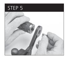
5. Insert ¼ – 20 X ¾ FLAT HEAD SCREW and tighten. *Do not use Loctite*®.
