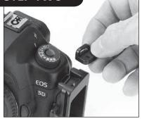
2. Insert CAMERA STRAP CONNECTOR into the top of the L-BRACKET.
