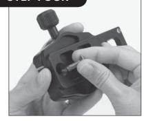
4. Apply **LOCTITE** to the threads of the second screw and insert it through the bottom of the bracket. Finger-tighten the second screw
