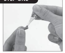
1. Apply LOCTITE on one of the STAINLESS STEEL SCREW
