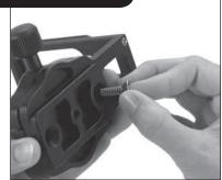
Line up the QUICK RELEASE clamp on the L-BRACKET and insert screw. Finger-tighten the screw in the QUICK RELEASE CLAMP.
