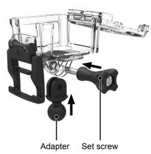
2. Place the Action Cam inside the standard housing, and press the lock downward until it locks tightly.
