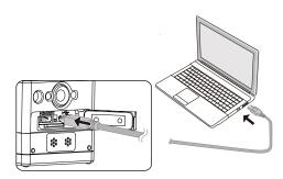
2. Open the Action Cam folder on the computer to copy your files to the computer. After the transmission is completed, please unplug the USB cable in a safe manner according to the computer's settings.
