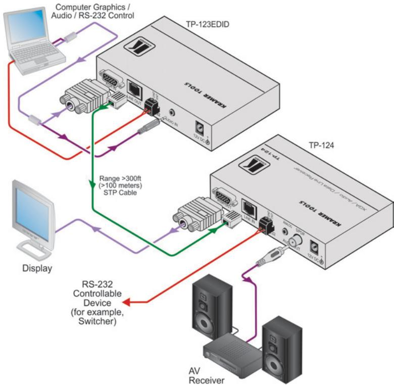
Figure 4: Connecting the TP-123EDID XGA/Audio/Data Line Transmitter
