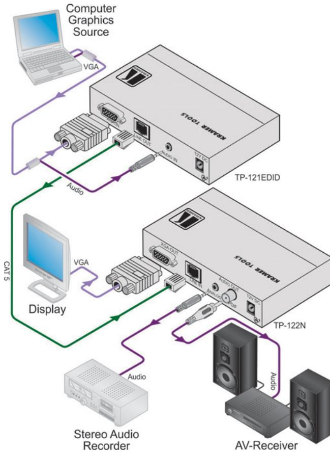
Figure 2: Connecting the TP-121EDID XGA/Audio Line Transmitter
