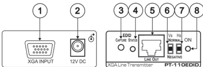
Figure 9: PT-110EDID XGA Line Transmitter
