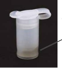
The tiny vial is about 1/2 inch tall and contains 25 mg of silver paste.
