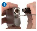
If the sleeve is pulled down and covering the connector, squeeze the end of the sleeve so you can feel the connector inside and press it into the jack until it latches.
