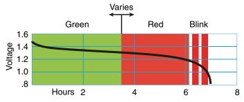
A weak battery will sometimes cause the PWR LED to glow green immediately after the transmitter is turned on, but will soon discharge to the point where the LED will turn red or the unit will turn off completely.
