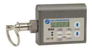
Hold the speaker on the RM close to the microphone when pressing the pushbutton. A "dweedle" tone will play from the RM speaker into the microphone and the parameter on the transmitter will be set immediately.
